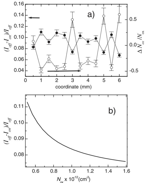
Fig. 5. (a) For different positions of the laser spot on unbiased n-Si sample ( $U = 0$ ) experimental SHG photomodulation efficiency (filled circles, left scale) and calculated  $N_{ox}$  (open circles, right scale). (b) Calibration of photomodulated SHG intensity vs the oxide trap density for n-type MOS structure (external voltage  $U = 0$ ) with the use of  $\eta(U)$  dependence plotted in Fig. 3(a).
