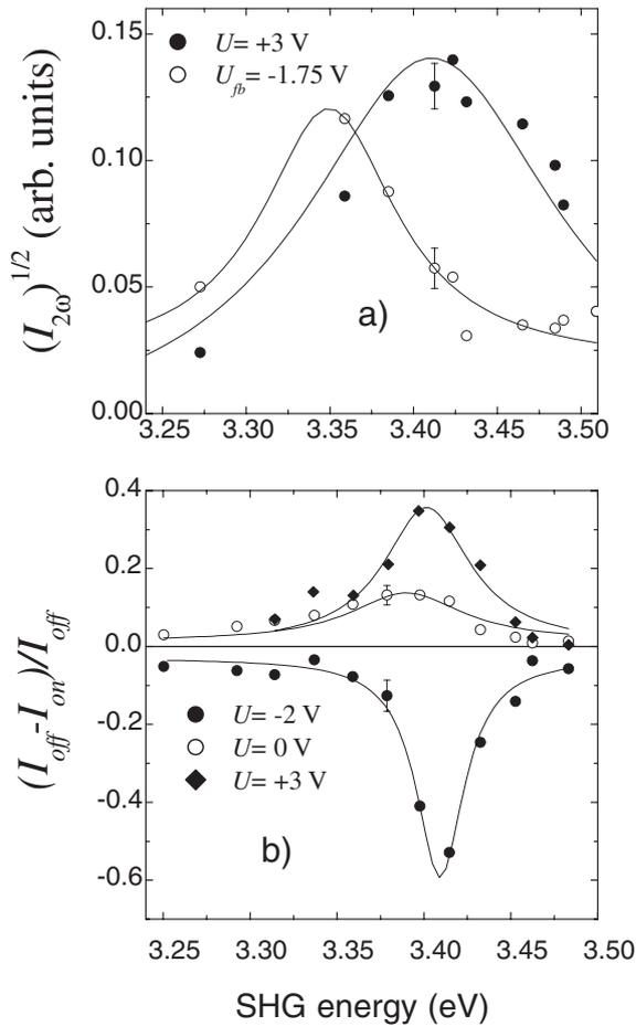
Fig. 4. Spectral dependence of the SHG intensity (a) and photomodulation efficiency (b) in p-Si MOS structure measured at different voltages. Lines—guide to eye.
