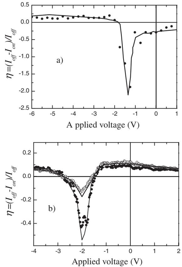
Fig. 3. The voltage dependence of the efficiency of the SHG photomodulation: (a) n-Si, average illuminating power 100 mW; (b) p-Si, average illuminating power 100 mW (filled circles) and 60 mW (open circles) Lines: model calculations. Experimental and model parameters are the same as in Fig. 2.
