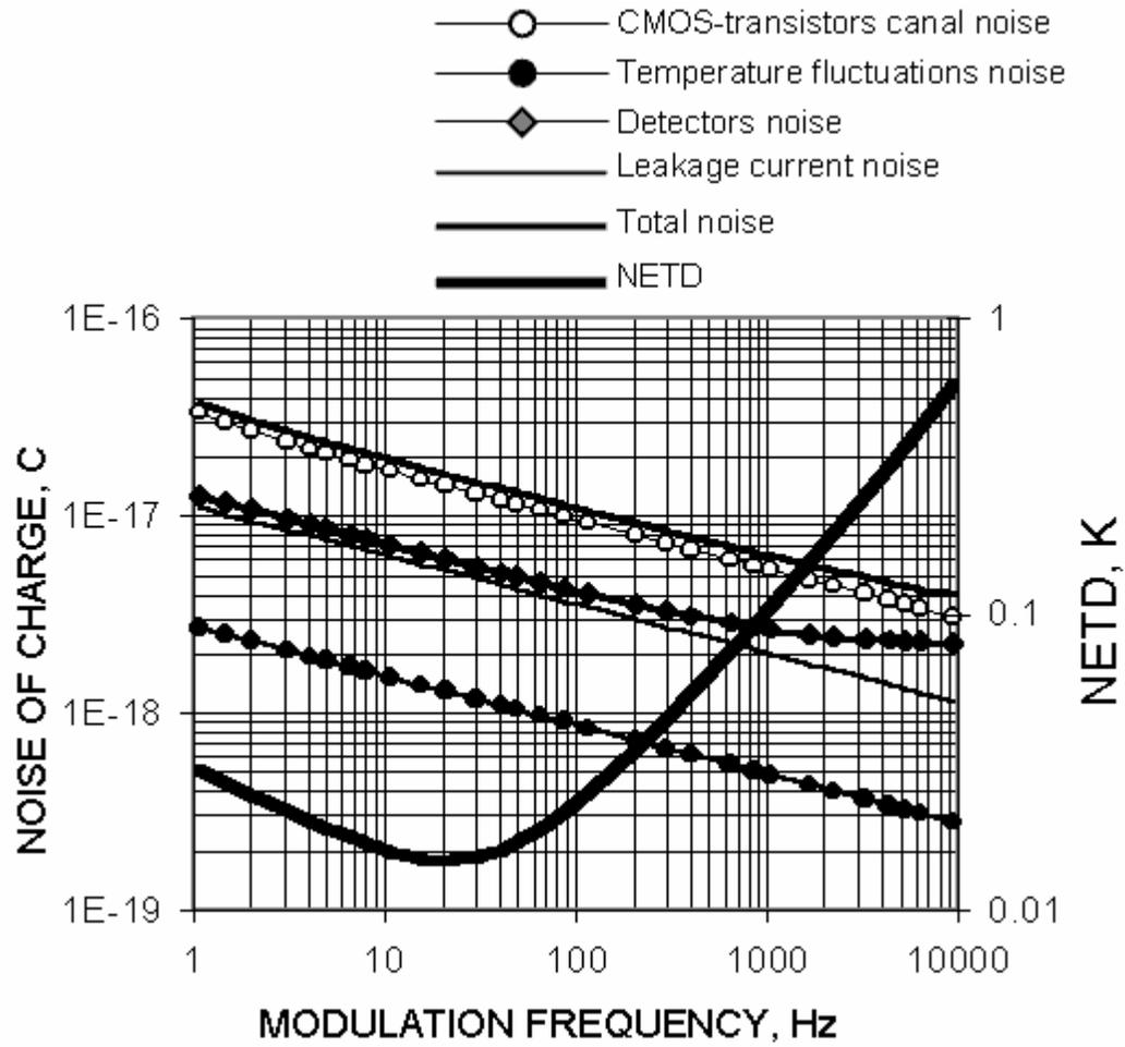
**Figure 2.** Calculated noise spectral densities and NETD of pyroelectric detector.
