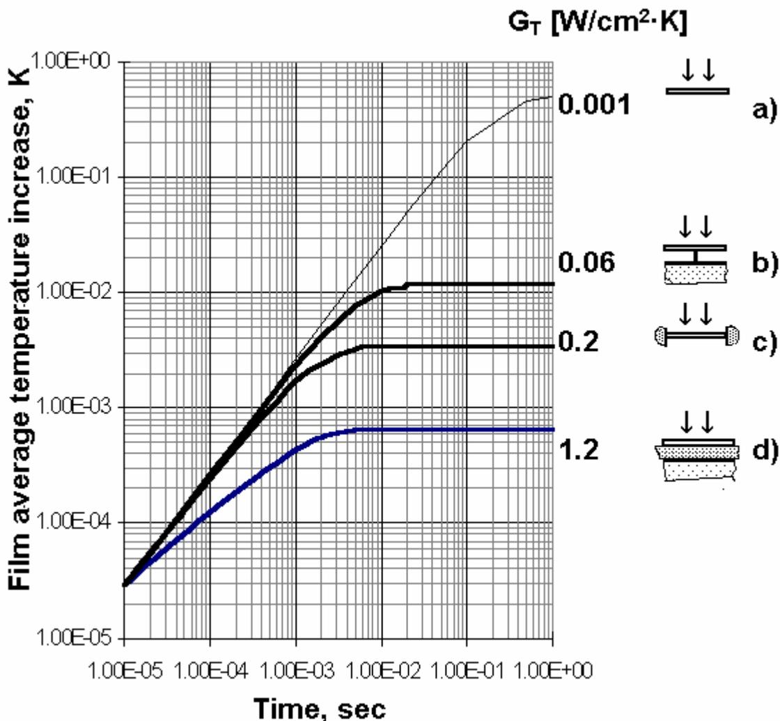
**Figure 1.** Mean temperature transition functions for different types of detector construction ( $1\mu\text{m}$  thick and  $\sim 100 \times 100 \mu\text{m}^2$  area) for different designs: isolated film in vacuum (a); heat sink of  $10\mu\text{m}$  diameter in the film centre (b); heat sink along the film perimeter (c); the film on a heat-insulating substrate of polyimide ( $10\mu\text{m}$  thick) (d).  $G_T$  is heat conductivity of the constructions.
