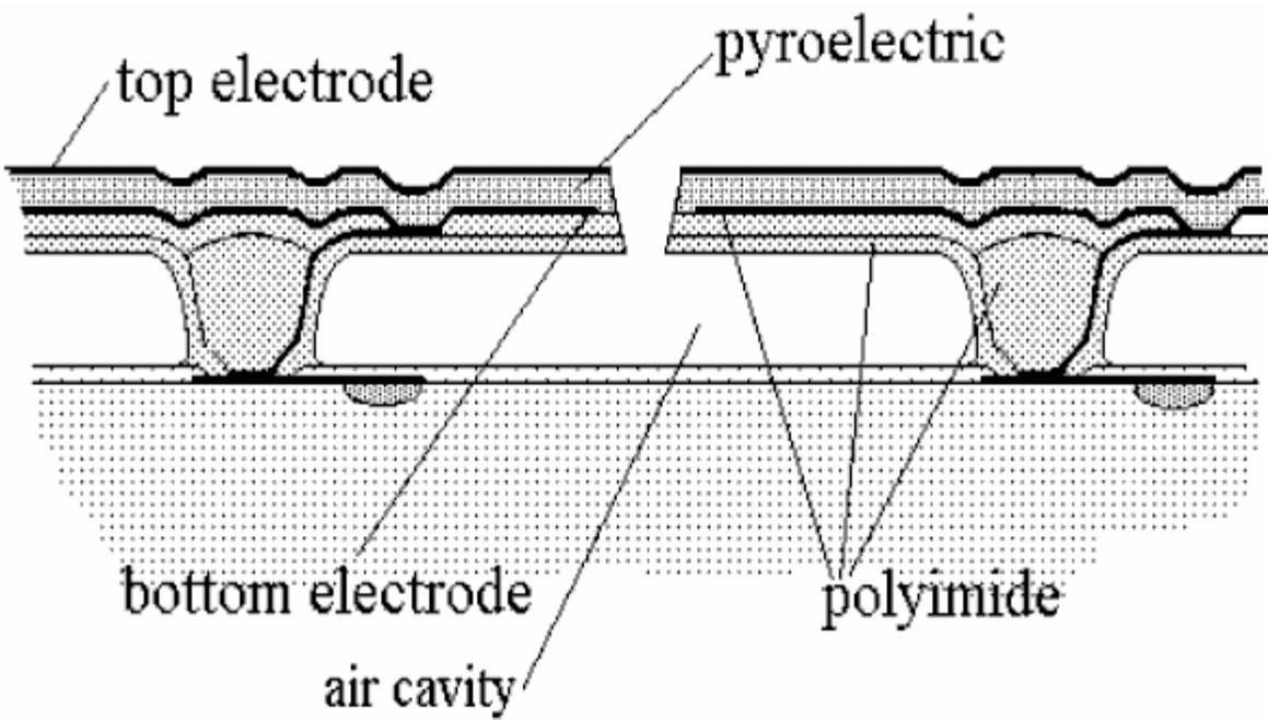
**Figure 3.** Schematic design of the multi-element integrated detector with polyimide membrane.
