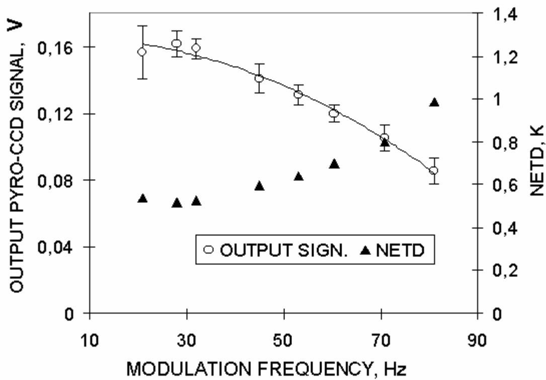
**Figure 4.** Output CCD signal vs. modulation frequency of incident IR radiation.
